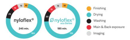
Overall 20% faster plate processing possible when using nyloflex® eco plates (in direct comparison to standard nyloflex® FAC).<sup>2</sup>
