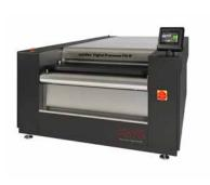
Premium quality incremental processor with pre-wash section for digital layer separation. The 3D brush motion system with servo driven motors automatically synchronizes the brush rotation and oscillation to the plate transfer speed, ensuring a constant and repeatable washout speed. Constant solvent temperature due to water circulation coil. Fresh solvent consumption control. Automatic solvent replenishment. Equipped with pinbar storage for up to 8 pinbars and automatic rollaway punching.
