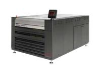
Compact all-in-one system, includes exposure unit for back, main and post exposure, batch-washer, dryer and light finisher. Perfect for narrrow and mid web applications. 24 memory channels for processing parameters and PLC control. Exposure with 19 UV-A lamps, cooled bed and airflow. Batch washer with solid content measurement and automatic solvent replenishment. Drying section includes four drawers with individual timers.
