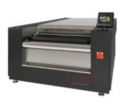
Premium quality incremental processor with pre-wash section for digital layer separation. 3D brush motion system with servo driven motors automatically synchronizes the brush rotation and oscillation to the plate transfer speed, ensuring a constant and repeatable washout speed. Fresh solvent consumption control. Automatic solvent replenishment. Delivered with a stand-alone punching device. A constant solvent temperature due to water circulation coil.
