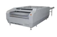
Digital washer with flat and round brushes in mid-size format. Equipped with double tank which allows to separate the black layer of the digital plates from the washout solvent. Automated brush height setting for optimum brush pressure according to the plate thickness. Temperature control of the washout solvent and integrated solid content measurement.
