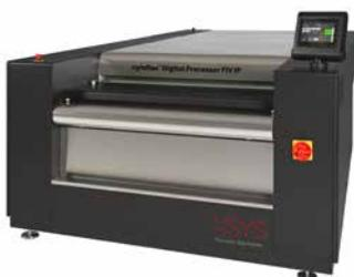
Premium quality incremental processor with pre-wash section for digital layer separation. The 3D brush motion system with servo driven motors automatically synchronizes the brush rotation and oscillation to the plate transfer speed, ensuring a constant and repeatable washout speed. Constant solvent temperature due to water circulation coil. Fresh solvent consumption control. Automatic solvent replenishment. Equipped with pinbar storage for up to 8 pinbars and automatic rollaway punching.
