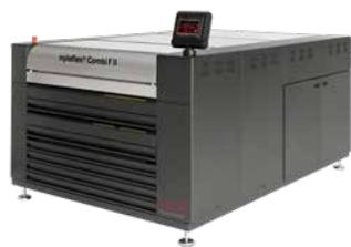
Compact all-in-one system, includes exposure unit for back, main and post exposure, batch-washer, dryer and light finisher. Perfect for narrow and mid web applications. 24 memory channels for processing parameters and PLC control. Exposure with 19 UV-A lamps high power lamps, cooled bed and airflow. Batch washer with solid content measurement and automatic solvent replenishment. Drying section includes four drawers with individual timers.
