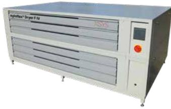
High powered heating output of 8.5 kW to quickly achieve the necessary operating temperature. Six drying drawers with high and wide opening. Two separate drying sections with individual temperature control for energy saving and efficiency provide uniform temperature distribution. Programmable digital timer for each drawer to allow the input of different drying times. Audio signal to indicate the end of drying time. Low energy consumption due to good heat insulation.
