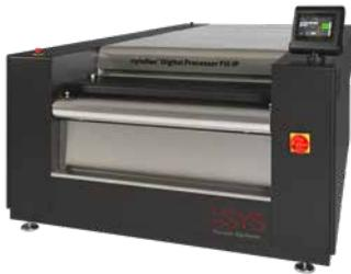
Premium quality incremental processor with pre-wash section for digital layer separation. 3D brush motion system with servo driven motors automatically synchronizes the brush rotation and oscillation to the plate transfer speed, ensuring a constant and repeatable washout speed. Fresh solvent consumption control. Automatic solvent replenishment. Delivered with a stand-alone punching device. A constant solvent temperature due to water circulation coil.
