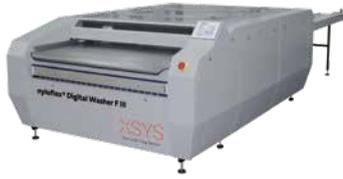
Digital washer with flat and round brushes in mid-size format. Equipped with double tank which allows to separate the black layer of the digital plates from the washout solvent. Automated brush height setting for optimum brush pressure according to the plate thickness. Temperature control of the washout solvent and integrated solid content measurement.
