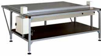
Designed for the cutting of foil based polymer plates up to 7 mm plate thickness (before and after processing) . The cutting blade and clamp is operated by compressed air. With illuminated cutting channel for best cutting accuracy, cutting angle 90 °. With two-handed operation for optimum work safety.
