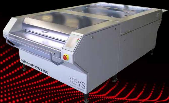
**Large-size flowline combination, suitable for processing water washable printing plates up to a maximum width of 1000 mm (39.4")**
